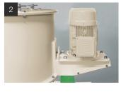
The frequency controlled drive brings the centrifugal disk up to 3.600 revolutions per minute.
