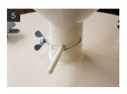
The desired throughput volume can be set precisely using a sliding gate valve.
